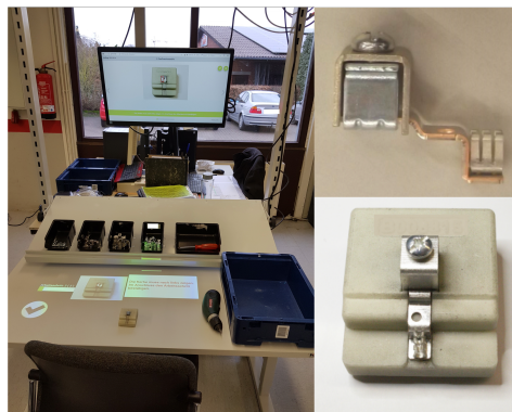
Fig. 3. View of the projection-based WAS in the vocational training area of the sheltered workshop (left) and the component to be assembled during the observations (right).
