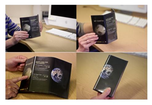
Fig. 4. Four views of a (prototype) folding tablet computer
