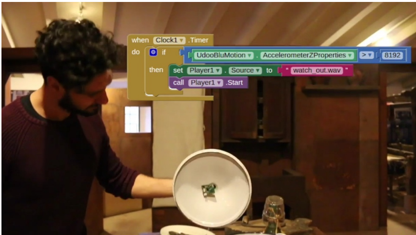
Fig. 8. Interactive cooking pot in the Sharecropping Museum. A. The setting. B. An UDOO Blu board is taped to the lid of a pot to detect its opening.
