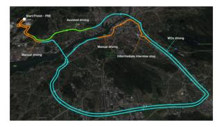
**Fig. 3.** The route of the test. Participants were instructed to drive manually or using assisting functionality for longitudinal and lateral support until notified by the car that autonomous mode was available. When in autonomous mode the car asked the participant to take over the driving three times during the drive to explore how and when the participant discovered the information given by the prototype interfaces. The test took about 1 hour and 15 minutes for each participant.
