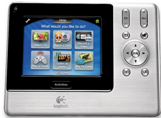
Figure 5. A “Universal” Remote Control. It is designed to alleviate the problem displayed in figure 1. This remote can acquire information about the units in a database (provided they are listed) and be programmed (through a computer) to perform the proper “key press” sequences, emulating the existing remotes on the living room desk. (picture from the web site of the Logitech company [12])
