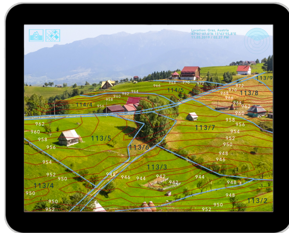
Fig. 5. Visualization of topographical contour lines and legal boundaries via augmented reality.
