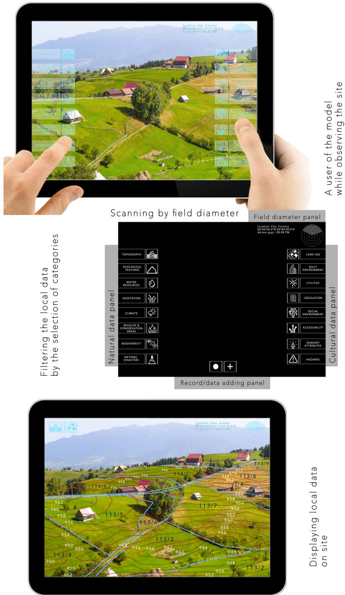
Fig. 3. User interface with tools of interaction for the model.
