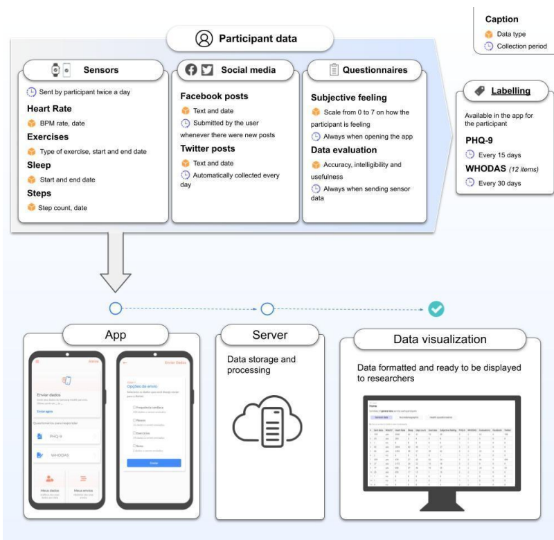
Fig. 1. Top: Data collected to build the computational model for the Amive project. Bottom: Modules implemented for data collection (App), storage and processing (Server), and visualization.
