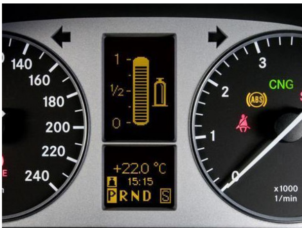
Figure 5 Mercedes Class B bi-fuel: panel cluster instruments, focus on the CNG indicator [source: www.metanoauto.com, consulted on 18/06/2008]
