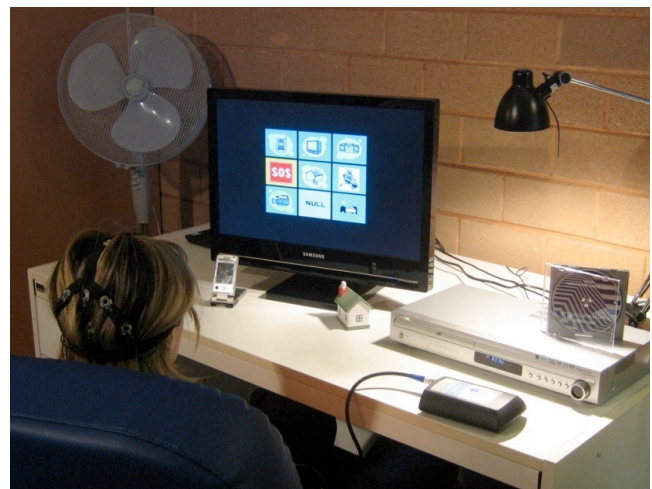
Figure 1. Prototype setup in which a P300-BCI control signal is utilized to control domotic appliances.
