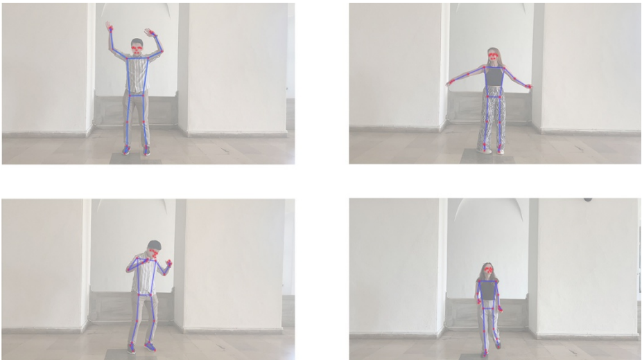
Fig. 4. Skeleton joint detection using the MediaPipe Pose library.
